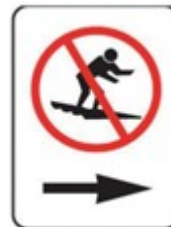
Figure 5 – Surfcraft Prohibition Signage (as shown in A/NZS 2416:2010.2)
